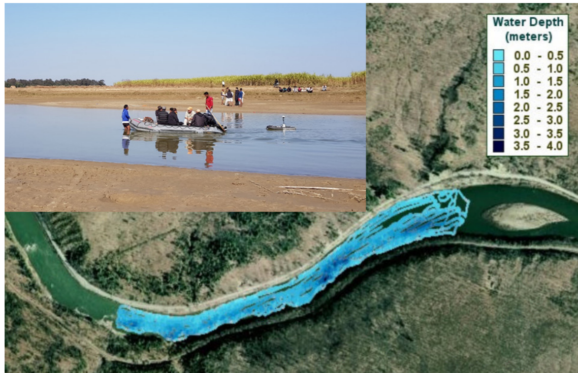
Figure 16. Bathymetric survey using acoustic Doppler Profiler and sonar trace of depth measurements
